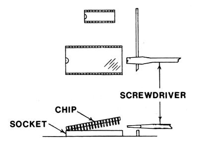
Figure 4. Removing the Video Control ROM Chip
