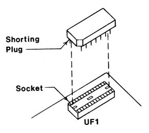
Figure 7. Orientation of Shorting Plug
